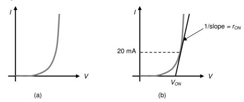
A tangent to the characteristic is now drawn such that this touches the line at the current to be used in the circuit. The slope of this line can be used to determine the effective resistance of the diode at this current, and the intersection between the line and the horizontal axis gives the effective ON voltage of the diode. (b) above shows this for a typical diode current of 20 mA.
