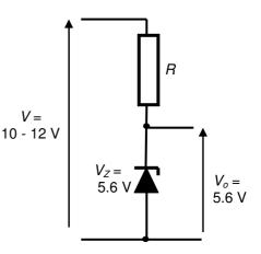
Maximum power dissipation in the diode occurs when the input voltage is at a maximum (12 V) and no current is taken by the load. Under these circumstances the voltage across the *R* is 12 - 5.6 = 6.4 V, so the current through *R* (and hence through the diode) is 6.4/44 = 145 mA. The power dissipation in the diode is this current multiplied by the voltage across the diode (5.6 V) so  $P_{max} = 815$  mW.
